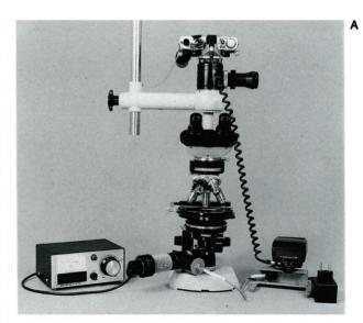
Obtaining the correct exposure involves a series of trials with neutral density (grey) filters, such that the light is attenuated to the appropriate intensity.
