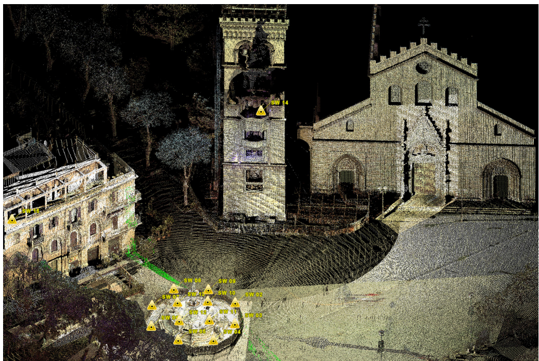
Fig. 10. Localization of the laser scanner station points on the entire point cloud of Piazza Duomo.
